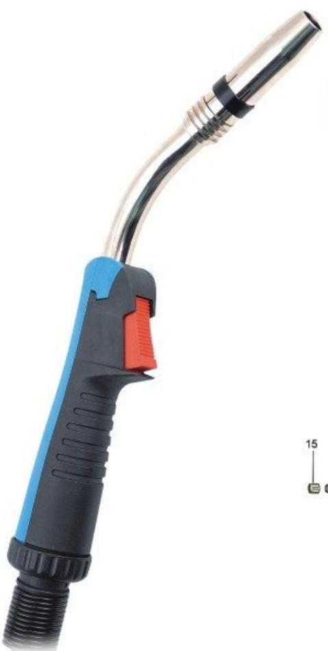
**40KD****Welding Gun c/w Euro Fitting**Rating: 350A CO<sub>2</sub> 320A mixed gas, 35% duty cycle.wires: 1.0-2.4mm
