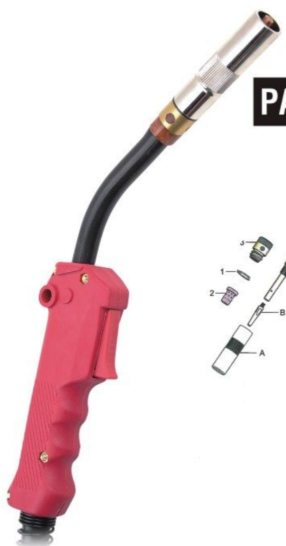
**PA500****Welding Gun c/w Euro Fitting**Rating: 500A CO<sub>2</sub> 420A mixed gas, 60 % duty cycle.wires: 1.2-1.6mm
