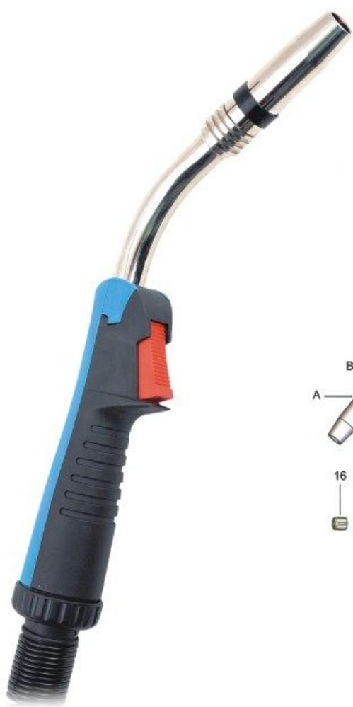
**24KD****Welding Gun c/w Euro Fitting**Rating: 250A CO<sub>2</sub> 220A mixed gas, 60% duty cycle.wires: 0.8-1.2mm
