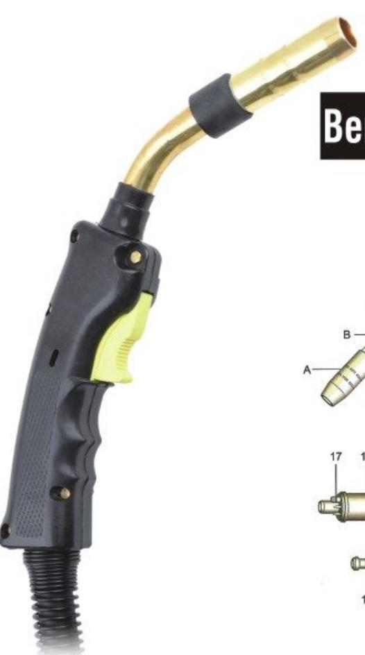
**Bernard200****Welding Gun c/w Euro Fitting**Rating:200A CO<sub>2</sub> 150A mixed gas,60% duty cycle.wires:0.03"-0.045"
